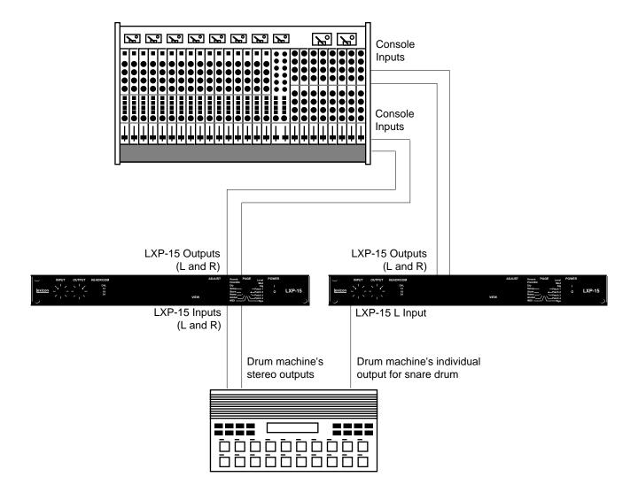
Using two LXP-15 units between your drum machine and console can make your drum machine sound much more exciting, since it allows you to process the all-important snare drum separately from the rest of the mix. Make sure you remove the snare from the drum machine's main stereo mix.
