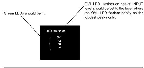
**Note:** If the OVL LED flashes with no input present it indicates processor overload is occurring.
