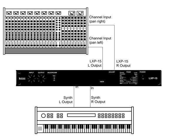
In some applications (such as when an LXP-15 is used for a single instrument) it may be desirable to patch the LXP-15 between the instrument and console. This makes it possible to keep the LXP-15 up on stage with other MIDI gear, rather than in the console effects rack, making MIDI control much easier.
