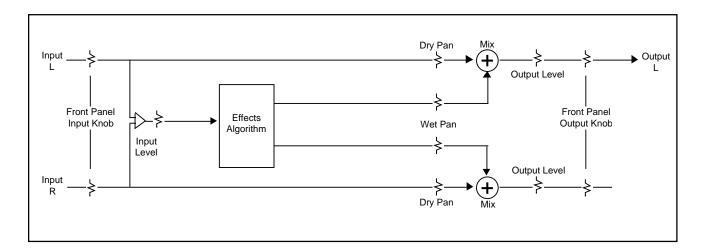
The routing and mixing of input and output signals for all algorithms are controlled by the five parameters found on the "Level" page. As these parameters are common to all LXP-15 algorithms, they are described first. The algorithm-specific parameters will be described with each algorithm.
