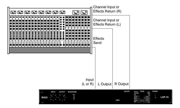
If you will be using an LXP-15 as your primary effects unit, and your system includes a console with one or more auxiliary (effects) sends, connect the LXP-15 as shown above. In most applications, it is preferable to connect the LXP-15 outputs to two of the console's input channel strips, panned full left and right, rather than the effects returns. This allows the greatest flexibility in routing and equalization.
