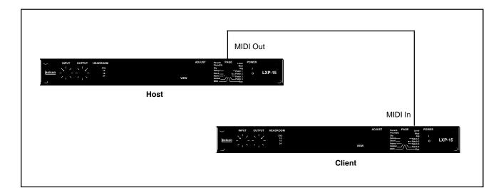
When connected in this way, the Client LXP-15(s) will be remotely controlled by the front panel of the Host as follows:
