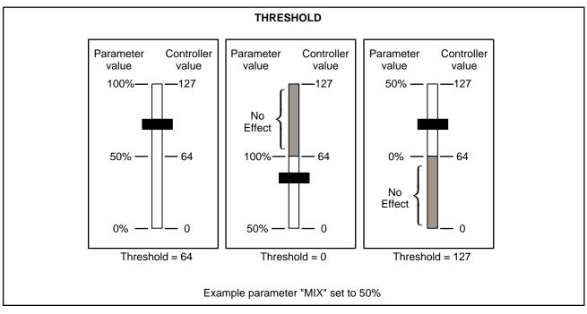
When using any of the Note Sources (LastNote, HiNote, LoNote), the threshold value is the *Note Number* that will correspond to the initial Destination parameter value. (On a standard 5-octave MIDI keyboard, 36 corresponds to the lowest C, 60 is middle C, and 96 is the highest key.) Threshold should be set to a value within the overall Note Number range of the MIDI controller.
