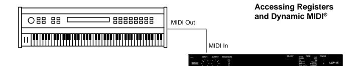
Some extremely useful effects can be created by controlling the LXP-15's variable parameters remotely in real time. Almost all of the controllers found on a MIDI keyboard or MIDI foot controller (pitch benders, mod wheels, sliders, switches, breath controllers, foot pedals and footswitches) can be used to adjust the LXP-15's parameters. We refer to this real time remote control capability as Dynamic MIDI<sup>®</sup>.
